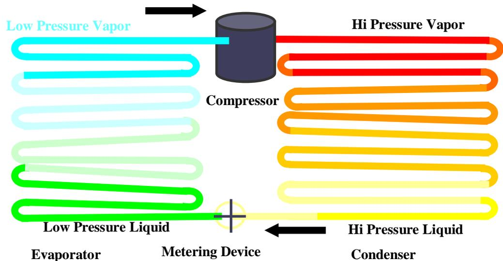
5. **The correct answer is (a) and (C). Transfers heat to the refrigerant from the indoor air and converts liquid refrigerant to gaseous refrigerant.**
