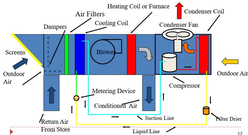
“Heat pumps”, were mentioned earlier as “reverse cycle air conditioners”. If one installed an arrangement of valves that allowed the refrigerant flow to be redirected so that the evaporator became the condenser and vice versa, our air conditioner would remove heat from the outdoors and transfer it to the indoor air. This is exactly how a heat pump operates.
